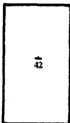
Figure 92. No-Bottom Sounding. The symbol represents soundings for which true depths have not been determined. The value indicates the depth sounded without bottom being struck.
